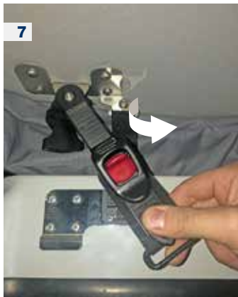
7 Rotate the complete freed ratchet system upwards towards the roof.
