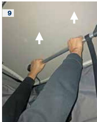
9 Grab the handle with both hands and push the upper part of the roof in upward direction.
