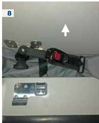
7 Rotate the complete freed ratchet system upwards towards the roof.
